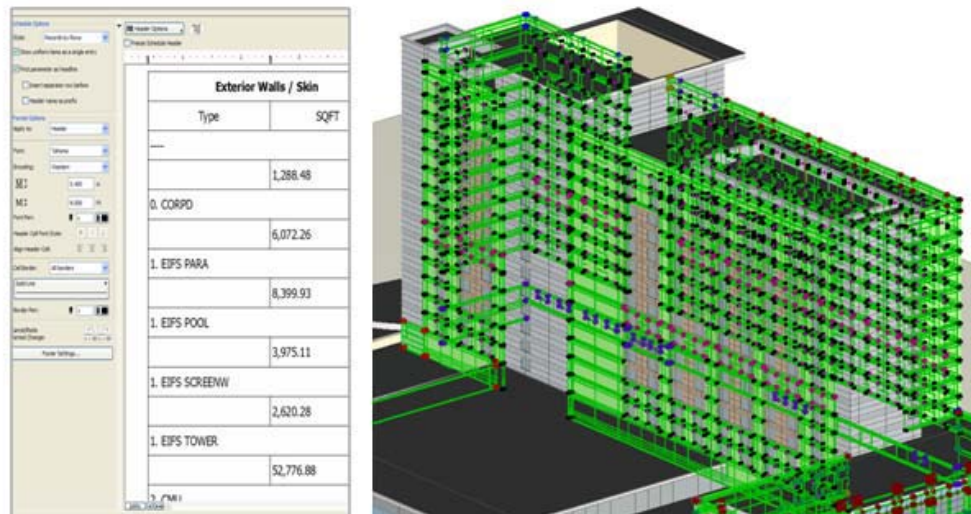
Figure 2.5 Quantity take off from building model (Note: This is not the Psychology Building).
